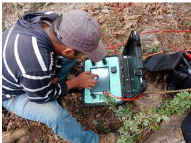
Seismic Refraction survey at Upper Arun HEP
